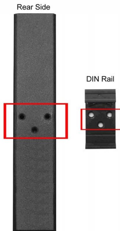
1. Use the screws to screw the DIN-Rail on the rear side of the industrial switch.
