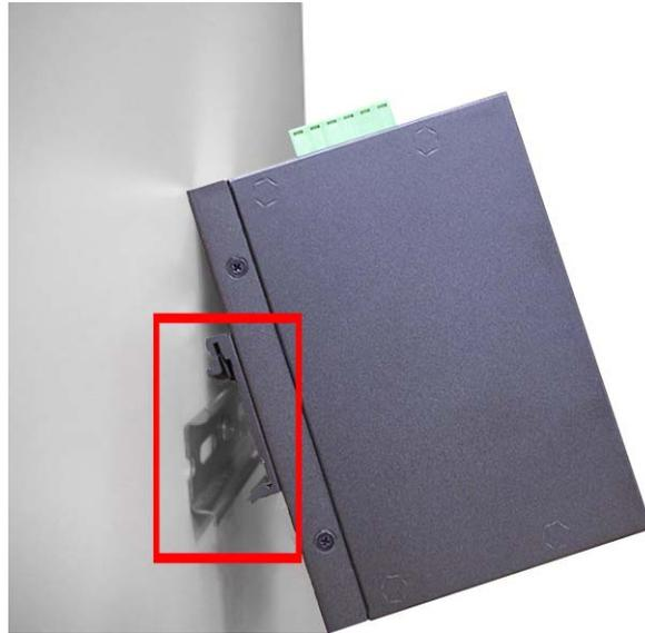
4. Then, lightly push the DIN-Rail into the track.
