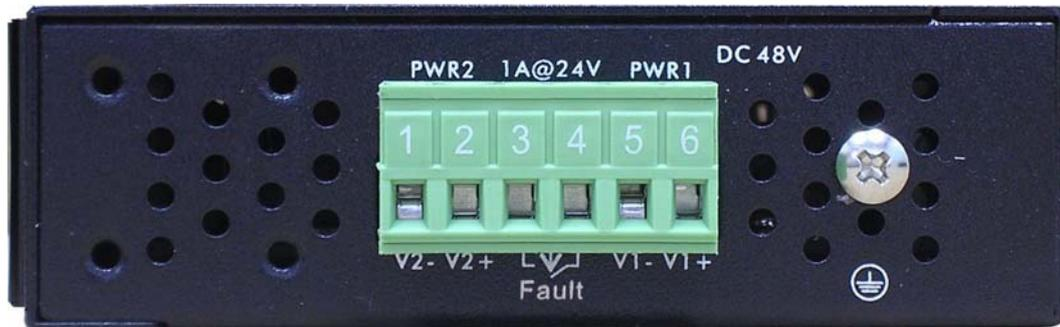
Top View of the PoE Injectors Industrial Switch
